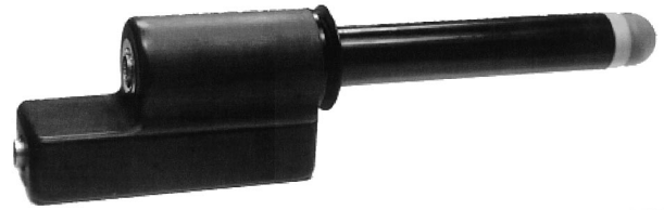
Fig. 2. The transvaginal 3-D probe. Dome length: 175 mm, total length: 298 mm, dome diameter: 25.6 mm, transducer center frequency: 7.5 MHz. The probe had no external moving parts except for the cable connector.
