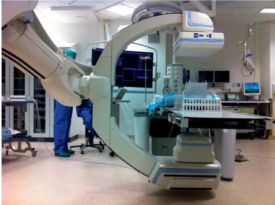
Figure 1.8: The C-arm Artis zeego from Siemens Healthineers (Erlangen, Germany) during imaging of an accuracy phantom. The C-arm is integrated with a floor-mounted robotic arm, which makes it very flexible, and can produce CT-like 3D volumes in addition to ordinary real-time fluoroscopic images.
