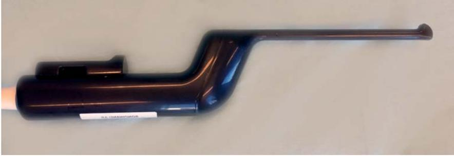
Figure 5.3: Prototype ultrasound probe for pituitary and spine surgery with a curved array, which allows for imaging to the side and forward at the same time.
