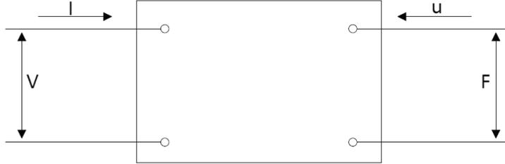
Figure 2.2: Electrostatic transducer modelled as a two-port network.
