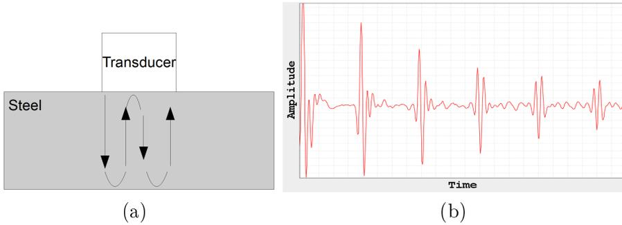
Figure 1.1: a) Typical setup for measuring wall thickness. b) Received waveform.
