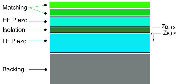
Figure B.2: Dual-layer transducer stack with the LF frequency element placed behind the HF elements
