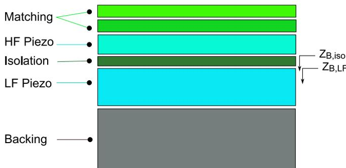
Figure C.1: Dual-layer transducer stack with the LF frequency element placed behind the HF elements [25]
