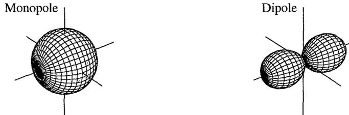
**Figure 2.1.** Scattering diagrams for monopole and dipole scatter. Scattered intensity as function of angle for a plane sound wave.
