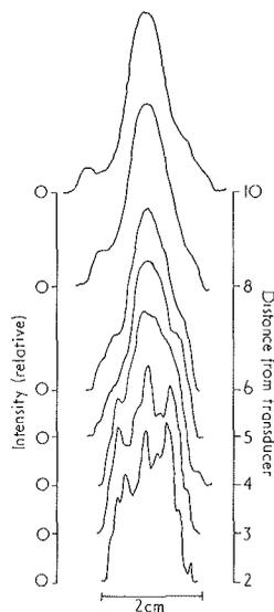
FIG. 7 Ultrasonic field intensity (relative) measured at different distances from an unfocused circular transducer of 18 mm diameter. Ultrasonic frequency is 2 MHz.
