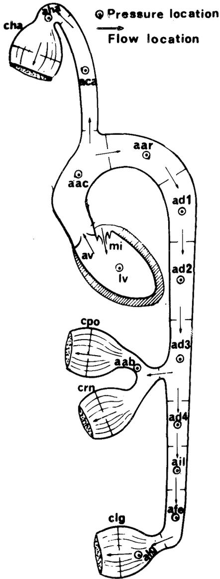
FIG 1. Model of the left ventricle and arterial system, showing the segmentation and the locations for measuring pressure and flow. Abbreviations: aac-ascending aorta, aar-aortic arch, ad1-ad2-thoracic descending aorta, ad3-ad4-abdominal descending aorta, ail-iliac arteries, afe-femoral arteries, alg-leg arteries, aca-carotid arteries, aha-head and arm arteries, aab-abdominal arteries. The abbreviations with suffix c (cha, clg, crn, cpo) signify the peripheral resistances.
