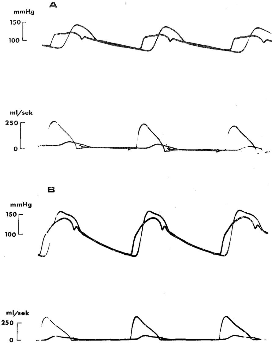
FIG. 3. Pressure and flow pulses in the aortic arch and the iliac artery of the model.
