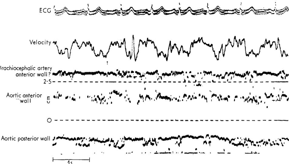
*M-scan of the aortic diameter measurement, using position B in Fig. 4. From top to bottom: ECG, velocity signal, and echoes from arterial walls; the upper echo is nearest to the transducer. The lower echoes represent the aorta, while the upper two lines represent an artery where the bloodstream was directed towards the transducer, probably the right brachiocephalic artery.*
