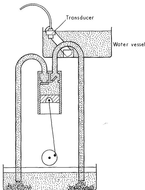
FIG. 2 Pump model for simulating pulsatile flow. The pump gives a constant stroke output, but stroke rate can be varied.
