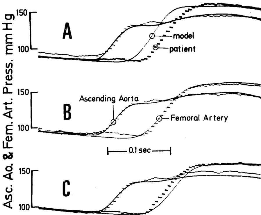
FIG. 4 Patient and model aortic ascending and femoral artery pressure at different values of aortic compliance in the model. In panel A the compliance is 0.55, in panel C 0.94 and in panel B 0.72 ml/mm Hg.
