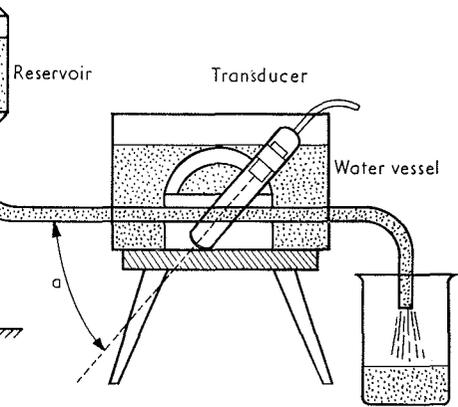
Experimental setup for testing the accuracy of velocity measurement. The reservoir is kept at a constant level from the ground by means of a spring. The angle between the transducer and the pipe ( $\alpha$ ) is varied.
