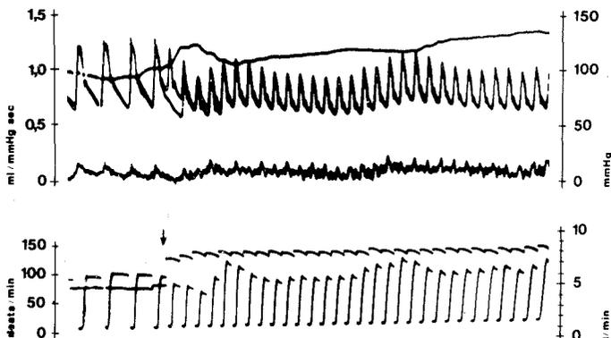
Figure 30.4. Cardiovascular parameters estimated during the Valsalva manoeuvre. From top to bottom are patient and model aortic pressure curves superimposed, peripheral conductance, pulmonary artery pressure and heart rate. The height of the vertical bars at the bottom of the figure represent cardiac output.
