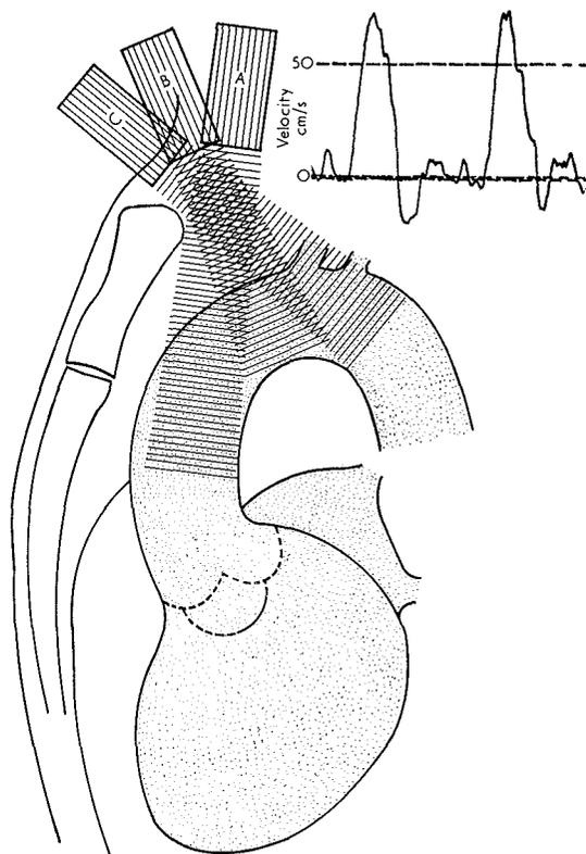
FIG. 4 Transducer positions for measuring aortic blood flow velocity in the aorta (lateral view). In position A and C, the velocities are measured in the ascending aorta and the aortic arch, respectively. In position B, the beam is normal to the blood stream, this position is used for measuring aortic diameter. The velocity in position A is shown on the right.
