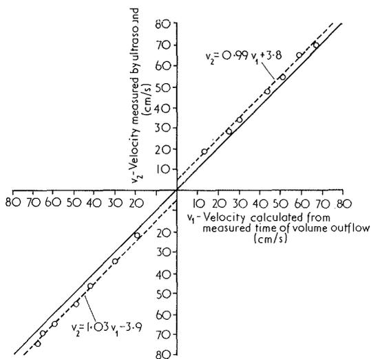
FIG. 6 Relation between velocities measured by ultrasound and calculated from measured time of volume outflow, using the experimental setup shown in Fig. 3. The line of identity is drawn. The high pass filter cutoff frequency is 200 Hz.
