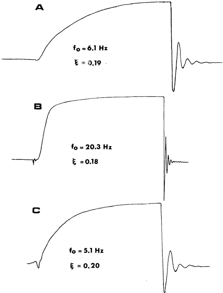
FIG. 1. The frequency response and dampening of a catheter-manometer system tested with the pop method (11). The frequency response and dampenings are calculated according to Gabe (11).
